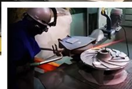
"SWING" system that allows ANGLE of the grinder at 0-90° facilitating the angular attack on the part.
